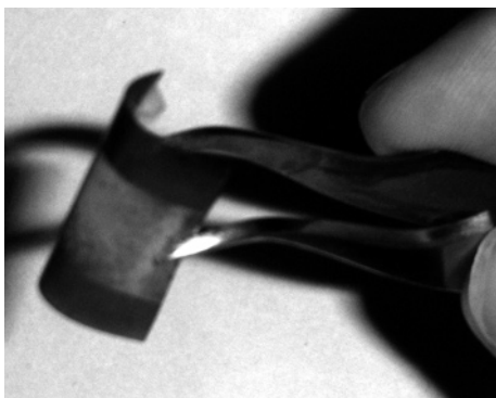
Figure 8. Photograph of a sample identical to Figure 7b, demonstrating excellent mechanical flexibility even after thermal treatment. The sample was heated at 300 °C for 3 h under ambient air.
